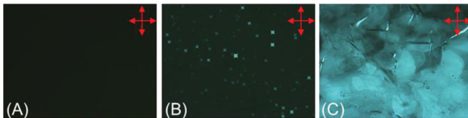
Figure 2. POM images of HO-biphenyl-O-CO-C 14 H 29 at 124.0°C (A), 113.5°C (B), and 105.5°C (C). Cooling rate is 3°C min -1 with magnification objective of 50×.
